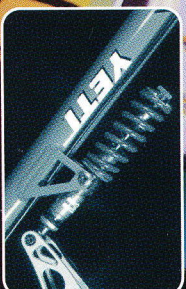
ROCK SHOX Coupe Deluxe pull-shock with separate coil-over spring preload and adjustable damping for fully-active, stiction-free travel.
