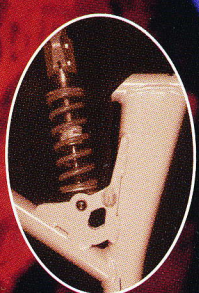
ROCK SHOX Coupe Deluxe shock with separate coil-over spring preload and adjustable damping for fully-active, stiction-free action.
