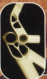
Extruded unibody bottom bracket and chain stay yoke work together to eliminate lateral flex at the lower pivot.
